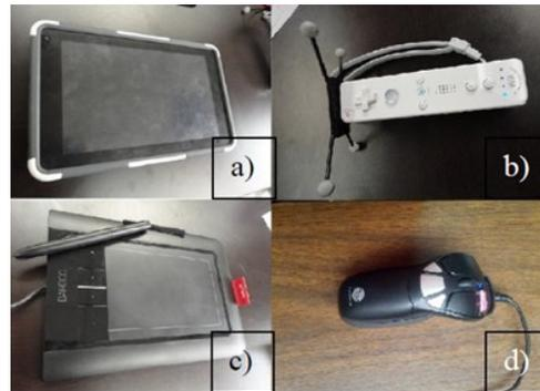
Figure 2. Input devices: a) G-Slate android tablet; b) Wii-mote; c) Wacom touch-pad; d) Air-mouse
